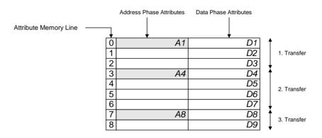
The figure shows three transfers, each one consisting of one address phase and several data phases. There is one column for the attributes for address phases, and another column for the attributes for data phases.
