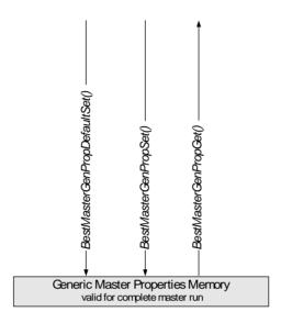
The generic master properties are not programmed using a preparation register. The generic master property memory is simply programmed by ...Set () and ...Get () functions, so that no further description is needed.
