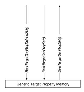
The generic master properties are not programmed using a preparation register. The generic master property memory is simply programmed by ...Set () and ...Get () functions, so that no further description is needed.
