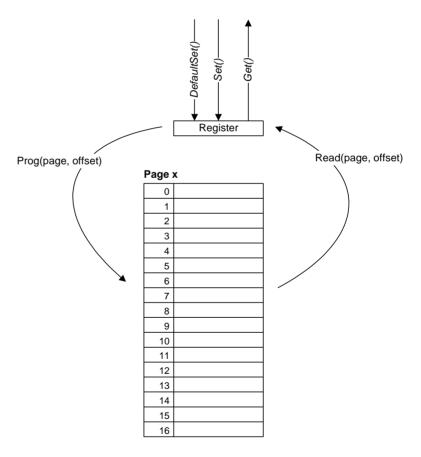
When programming a memory line with the content of the preparation register, a page pointer and a line pointer are passed with the referring command or function. These pointers are used to identify the exact memory line for reading and writing between the memory and preparation register.
