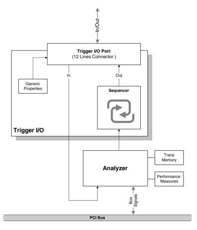
By programming the generic properties, you can specify which lines of the trigger I/O port are input and which are output. The **output** lines of the trigger port are controlled by a programmable sequencer. For more information on sequencers, refer to "Sequencer Programming" on page 55.
