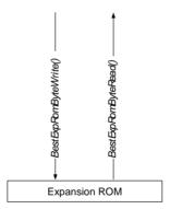
The expansion ROM is not programmed using a preparation register. The expansion ROM is simply programmed by ...Write() and ...Read() functions, so that no further description is needed.
