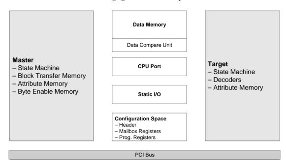
NOTE If master and target of the testcard are set up to transfer data from one to the other, the target has no access to data memory. If the master writes to the target, data memory will remain unchanged. If the master reads from target, it will receive dummy data.
