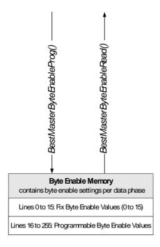
The byte enables are not programmed using a preparation register. The byte enable memory is simply programmed by ...Prog() and ...Read() functions, so that no further description is needed.
