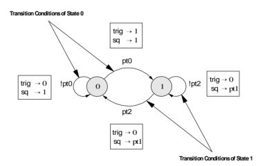
The example state diagram shows two states 0 and 1. Two transition conditions are used for state 0: pt0 and !pt0. State 0 represents the state before the first access to video memory. At this time all bus states are stored in the trace memory (storage qualifier set to 1, no filtering).
