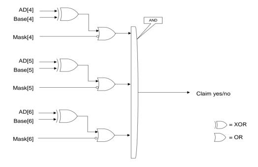
When decoding, the decoder compares the settings of address line, base address register and mask as shown in the figure. If the comparisons return "true" for all bits, the transaction will be claimed (if IDSEL and the bus command match as well).
