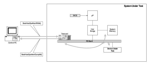
The testcard is plugged into a system under test and connected to a control PC.
