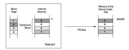
The PCI Protocol Permutator and Randomizer software internally permutates the different variation parameters of these blocks against each other to compute the required block page size, the last possible permutation using the specified block page size, and the estimated testing time. On demand, the block page can then be generated and downloaded to the testcard. The testcard can generate the traffic by executing that block page.
