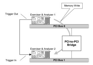
In the example, two testcards are needed. The testcards are placed on two PCI buses that are connected via the PCI-to-PCI-bridge under test. The testcards are set up for data transfer from one to the other, for example, with the Memory Write command.
